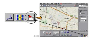
You can load scanned bitmap files as maps for in-building mapping, or use GSF and MIF map file formats for outdoor maps. Using GSF or MIF map files lets you use the built-in GPS receiver to automatically place measurements at your current location.
