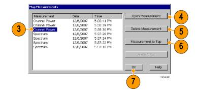
**NOTE.** You can also double-tap on a measurement icon to open the measurement window for that measurement. If there are multiple measurements at a location, double-tapping an icon displays the results for the measurement icon that is at the top of the list.
