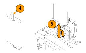
You can add a second battery to increase the operating time. Replace a battery with the specified type only. To purchase a battery, contact your Tektronix Service Center for the correct part number.
